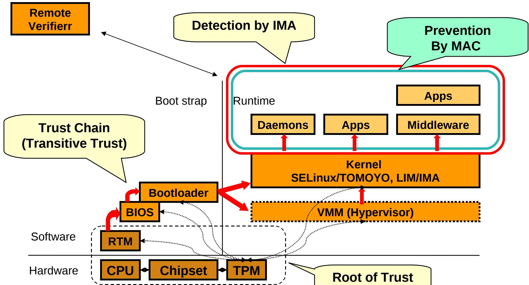
The platform (TCB) “integrity” is protected from software attacks and some hardware attacks (depend on security strength of HW)
